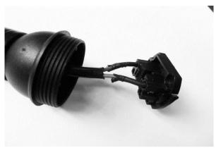
**■** 5. Connect wires to terminal in socket base
